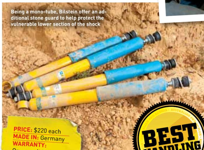
Being a mono-tube, Bilstein offer an additional stone guard to help protect the vulnerable lower section of the shock
