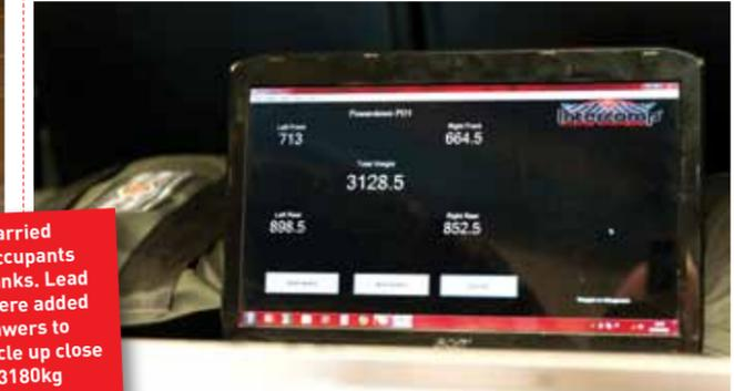
The test was carried out with two occupants and full fuel tanks. Lead weight bags were added to the rear drawers to bring the vehicle up close to the GVM of 3180kg
