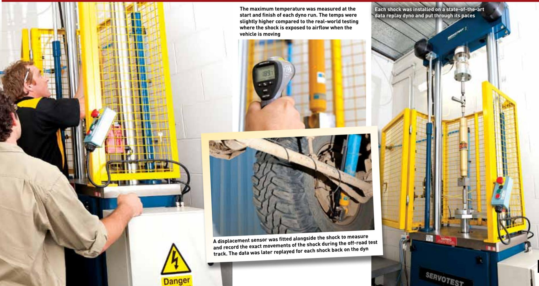
The maximum temperature was measured at the start and finish of each dyno run. The temps were slightly higher compared to the real-world testing where the shock is exposed to airflow when the vehicle is moving
